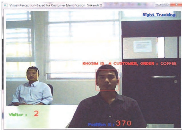
Fig. 14. Result of simulation using improved face recognition system and implemented to a service robot to identify a customer.
