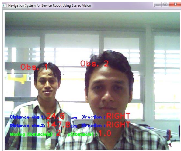
Fig. 9 The distance estimation for multiple moving obstacles using stereo vision.
