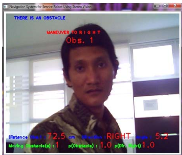
Fig. 10. The Distance estimation and direction estimation using stereo vision and implementation of probabilistics robotics for multiple moving obstacles avoidance.
