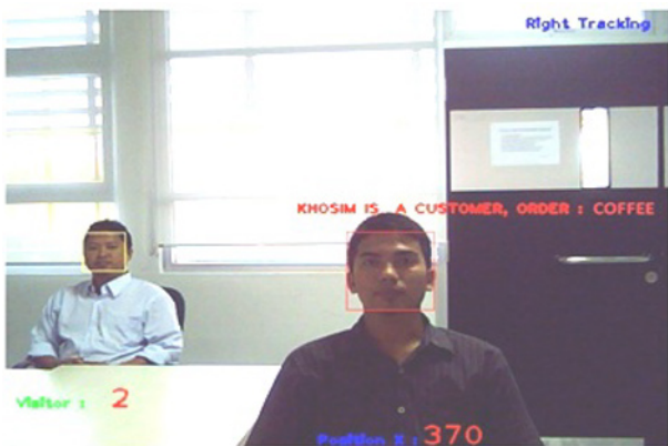
Figure 13. An example of face detected and recognized successfully using Haar Cascade Classifier and the information of the ordered product.
