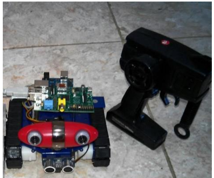
Fig. 6. 1 PING)))™ as distance sensor for obstacles avoidance and Minoru 3D stereo camera for robot[5].
