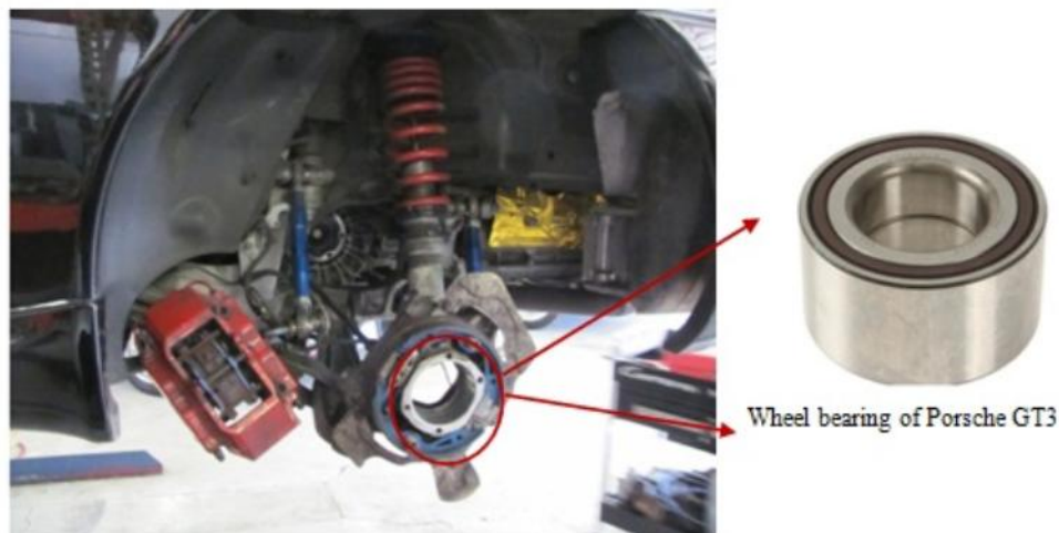
FIG. 1.1. Example of tapered roller bearing in automobile wheels
