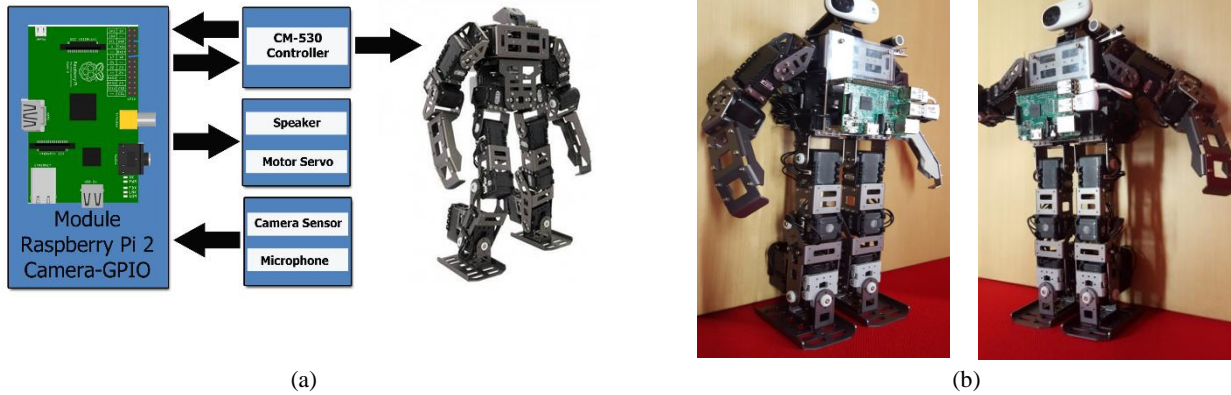
Fig.1. Our humanoid robot called as BeeHumanoid (a) robot architecture (b) side view appearance
