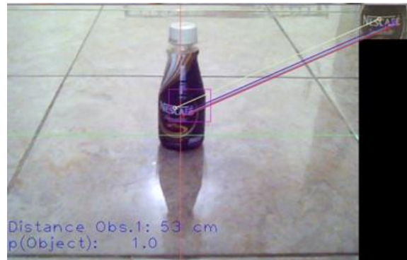
Figure 6. Robust Object detector using FLANN based matcher for manipulator, rectangle line used to get center position of the object.
