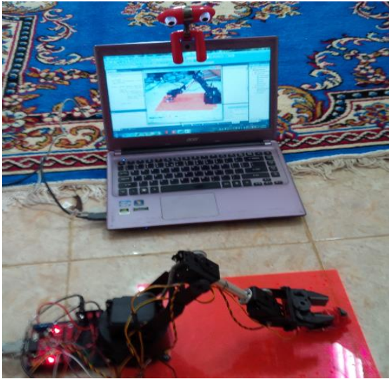
Figure 1. Proposed framework for vision-based grasping using Computer Vision and stereo camera at the side of the manipulator.
