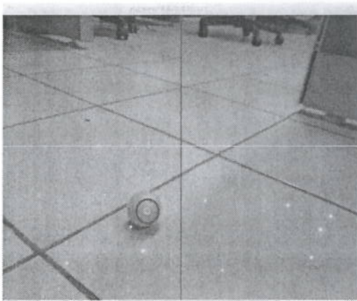
Fig. 6. The ball detected by our vision-based system for humanoid soccer robot.
